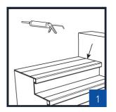
1. Finish seams with Quick-Step Coloured kit (QSKIT(-)) to hide any imperfections. The Coloured kit is available in white and different matching colours to your floor. The coloured kit is also paintable!
