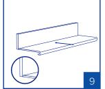
1. Measure the distance between the front of the Stair Cover and the below riser. < 46 mm: plank won't fit behind the Stair Cover. The bullnose must be enlarged or the Stair Cover adjusted to fit the floor plank for the riser and fully support the Stair Cover. ≥ 46 mm: check if you need to click an additional plank onto the bottomside of the Stair Cover to obtain a clean finish. Tape these two parts together on the backside and/or apply woodglue in the click profile.</p>
